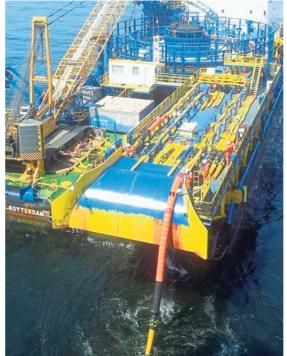
polyurethane will be bellmouths on the offshore substation foundation, protecting the interface of platform and export cables.
